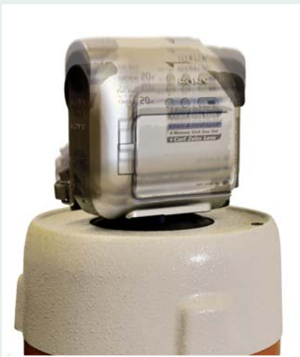
V406 shaker being used to test camcorder to ensure product reliability during operation.
